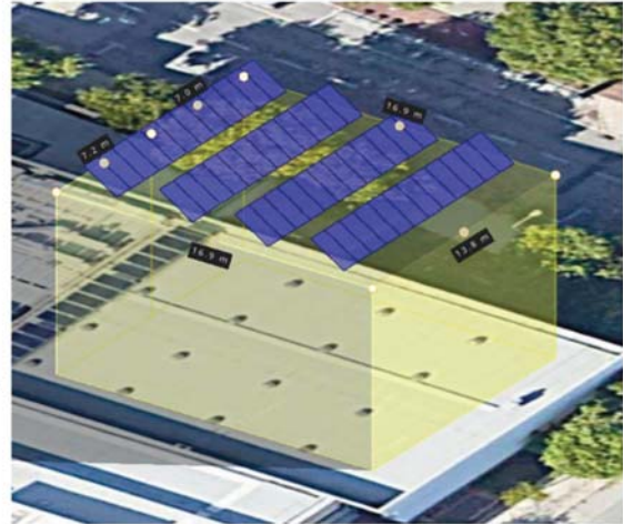
Figure 6.24 - Mira Rio School and Telheiras Church - S6 - A6 PV Simulation (HelioScope, 2023).
