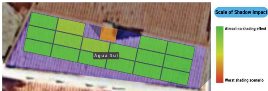
Figure 6.7 - Lagar of São Vicente's Farm - Shading effect on PV modules - Part A (HelioScope, 2023).
