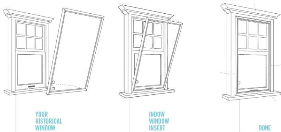
Figura 4.15— Sistema de storm window. ( https://indowwindows.com/solutions/insulating-drafty-windows/ .)
